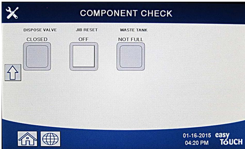
Pressing the home button to exit the function will display driving valves to ensure all valves return to home state. Once completed the controller will display FILL VAT FROM DRAIN PAN? YES NO. Press YES to ensure that any oil in the filter pan is returned to the vat.
