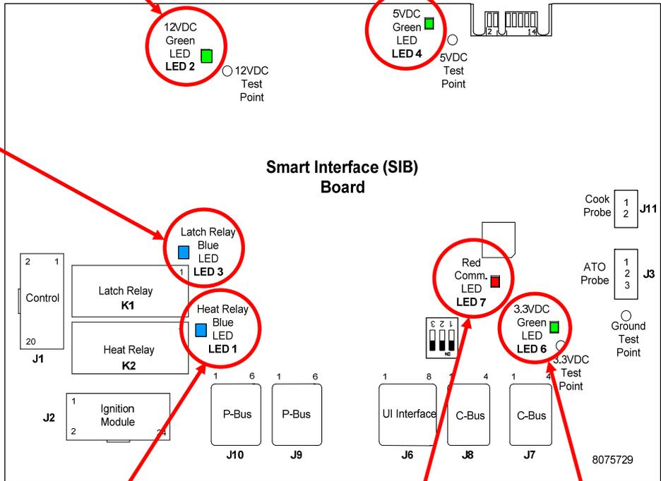
When UI calls for HEAT this LED will come on with the heat relay only after latch relay has been latched in and AIR switch has been proven. This LED will cycle with the call for heat.
