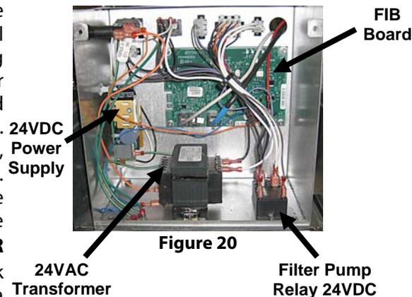
Press the information (?) button; press the down arrow; press the SW version button to verify software version of the FIB. If the FIB software version is not visible, the FIB may not be connected properly.
