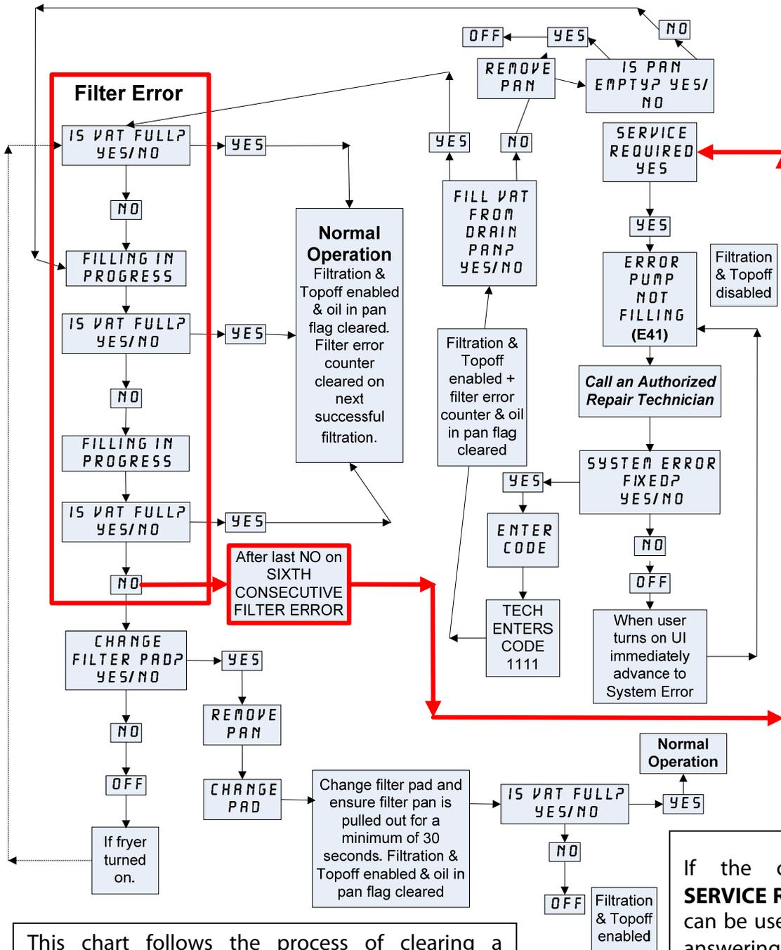
This chart follows the process of clearing a filtration issue. The prompt is displayed when any of the following occur:
